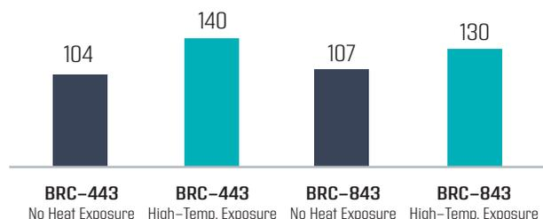
Figure 3. High Temperature Impact on Tensile Strength (psi)
