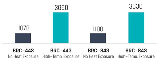
Figure 4. High Temperature Impact on Modulus (ksi)
